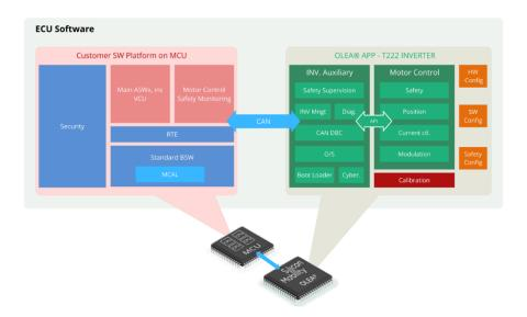
Alternatively, OLEA can be employed as a slave inverter controller, running the OLEA® APP – T222 INVERTER + ridge over CAN setup. In this capacity, it is viewed as a remote inverter controller, with speed and torque commands transmitted by a central VCU/VDU and the status and safety information collected by the same central VCU/VDU.
