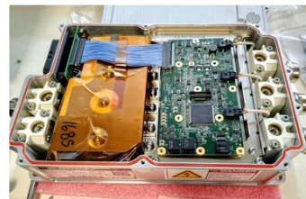
Figure 6: PM100DX inverter with integrated OLEA T222 FPCU based control board
