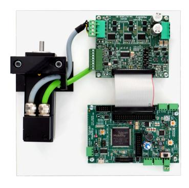
All-in-one hardware platform for a rapid start up of 3-phases PMSM motor control application using the best of OLEA® technologies.
